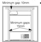
If you are going to install the appliance under a work counter, be sure to leave a 10mm space between the top and any other objects on or above the machine and a 15mm space between the sides and lateral furnishings or walls. This is to ensure
